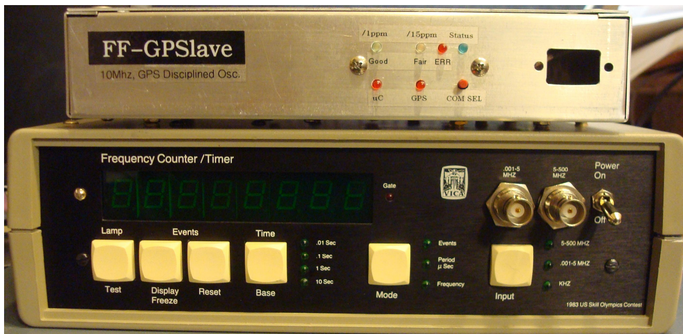
Figure 4. (Nearly) Finished GPS Disciplined Timebase and VICA contest Frequency Counter.
