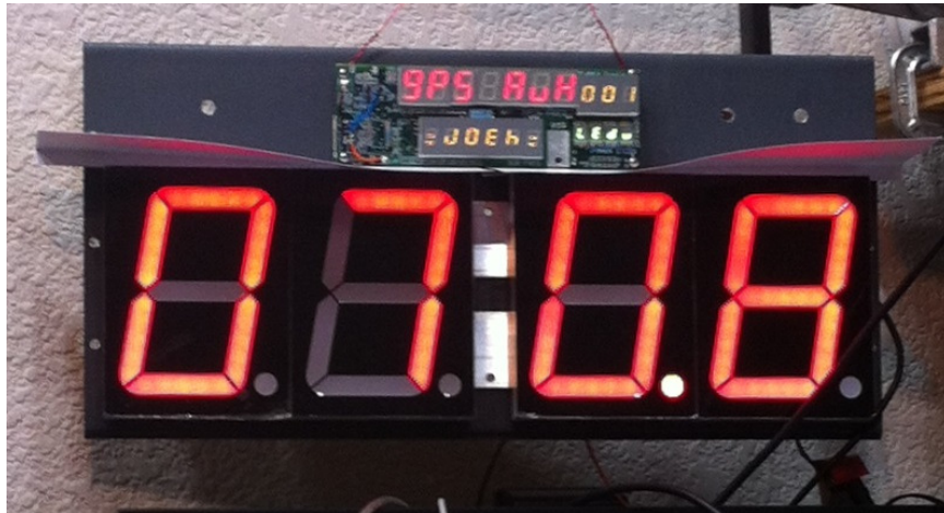
Early build stage of the clock internal frame (the central gap is for the not-yet installed colon section)
