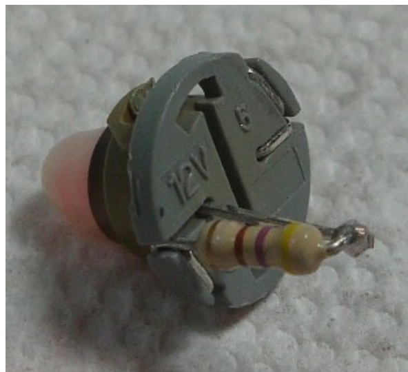
Unmodified lamp holder (left). LED-modified lamp holder (right) – the resistor is the (+) terminal.
