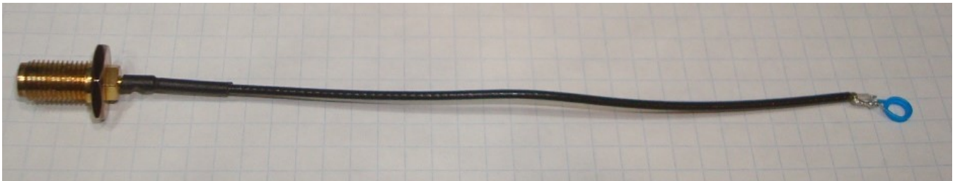
QTY One, MARK-I, regulation current/magnetic probe.
