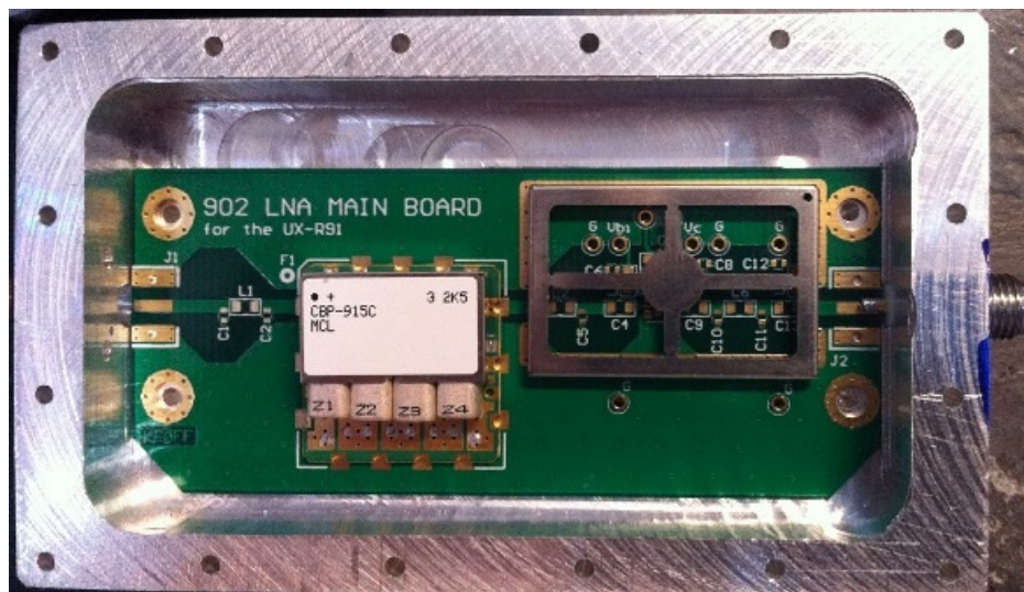
Figure 4. Fit-check of the LNA PCB inside the custom machined enclosure.
