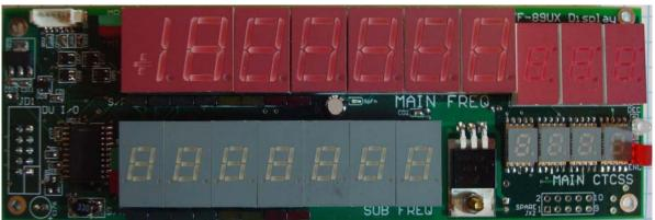
Figure 4. Display module, assembled
