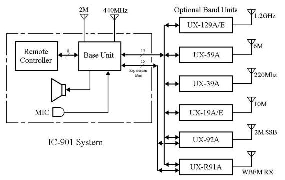
Figure 1. IC-901 simplified block diagram.
