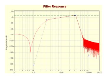
Figure 8. Quick Filter response for narrow-band FM shaping.
