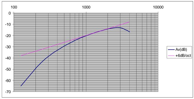
Figure 7. Measured frequency response of FM modulator circuit.
