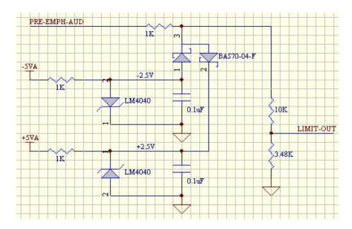
Figure 5. Revised limiter schematic
