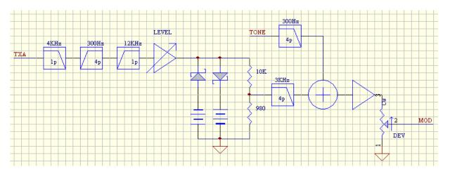
Figure 6. Final FM MOD filter chain for ICOM UX module
