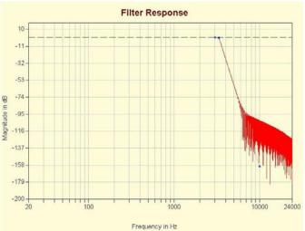
Figure 9. Quick Filter response for SSB shaping.
