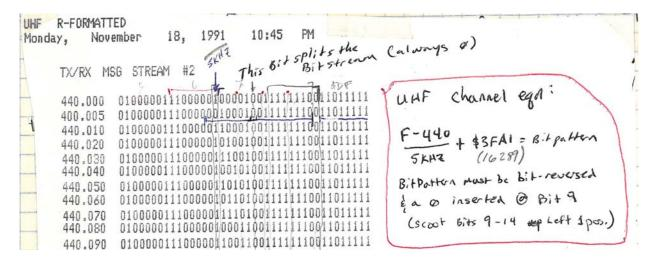
Figure 2. IC-901 data streams for the UHF unit. This print-out was edited to isolate the PLL bit fields.
