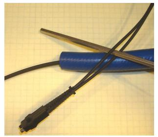
Figure 3. 3D housing mated to the FO cable and air-hose protective "conduit".
