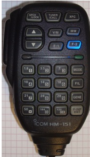
Photo 6. HM-151 LED shown illuminating the “F-2” button on an HM-151.
