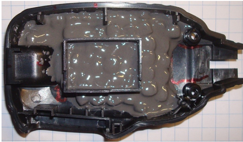
Photo 9. Final ballast configuration.
