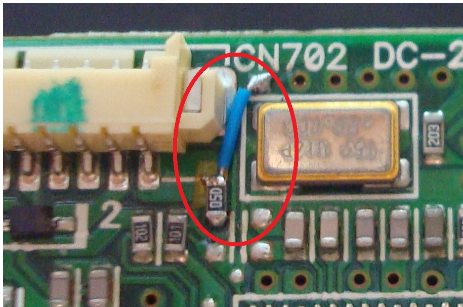
Photo 2. OVP extension resistor installation. Note: a layer of Kapton tape is placed under the chip resistor to prevent shorting to the underlying copper.
