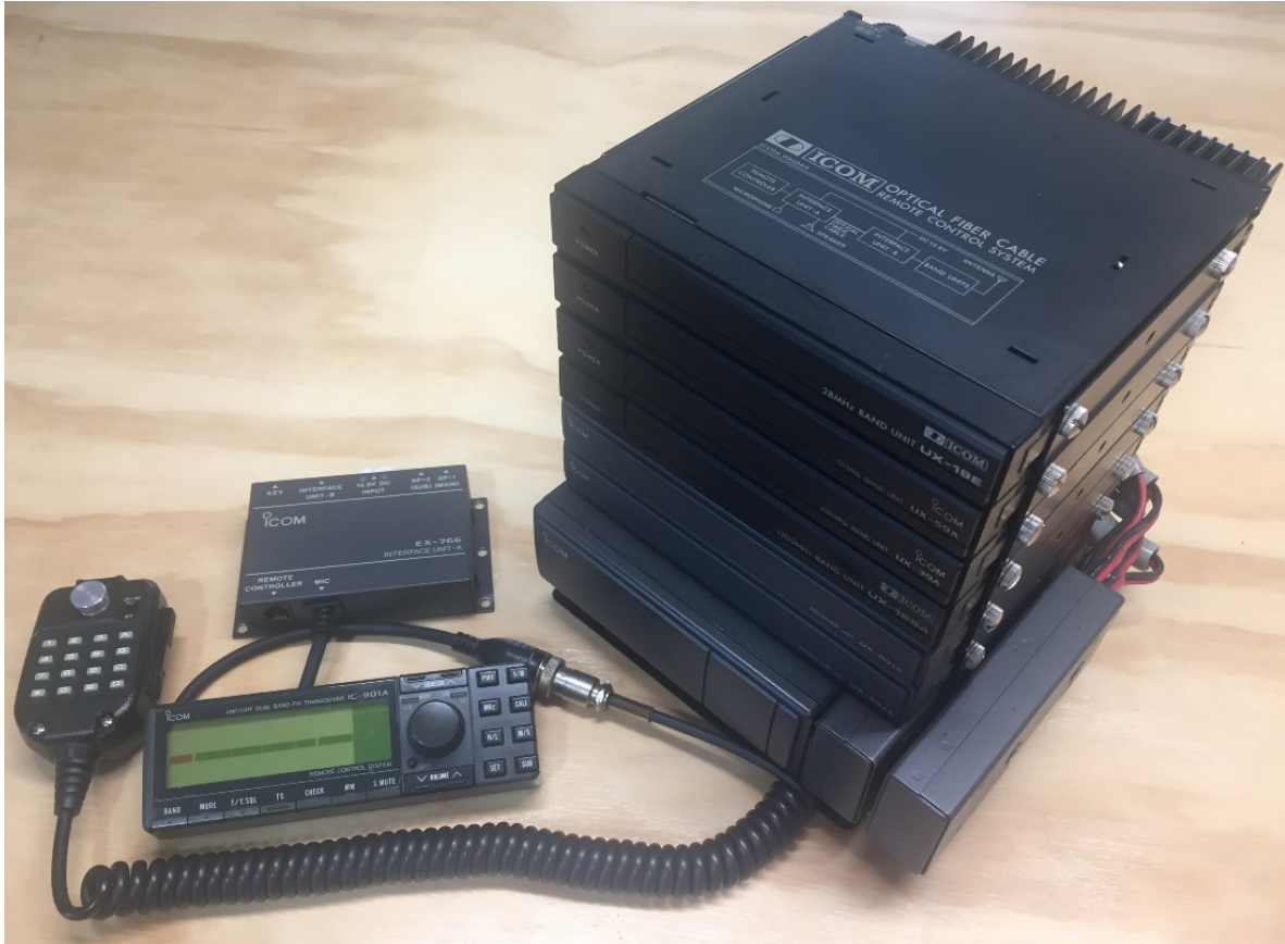
Photo 1. The essentials of a stock IC-901 system (minus cables). From left to right: HM-14 mic, Remote Controller, EX-766 Optical A-Unit, and an IC-901 Base Unit with a full compliment of RF modules.
