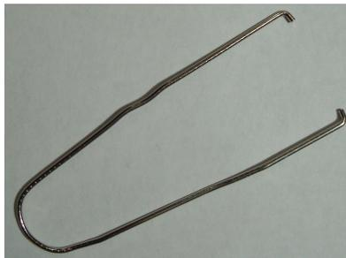
Figure 2. Paper-clip PCBA extraction tool. The gap should measure approximately 3/4”.
